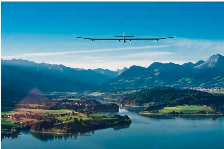
*Airborne adventure: the solar plane is scheduled to fly around the world without fuel. Bayer MaterialScience supports the "Solar Impulse" project with new material composites, helping to make the plane lighter and more stable.*
